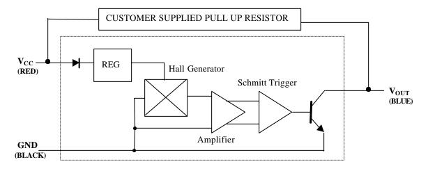
NOTE: A pull-up resistor is required on the open collector output to establish a quiescent voltage level. The pull-up resistor also provides faster rise times and improves noise immunity. Contact the factory for application assistance.
